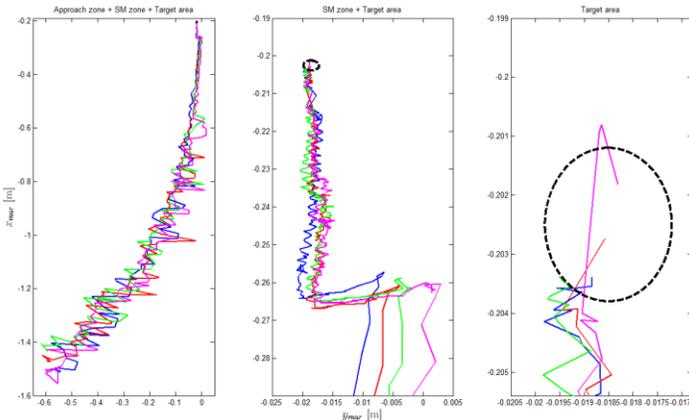
**Figure 4** Gain tuning for the designed controller in the autonomous vision-based docking (Alijani, 2016).
