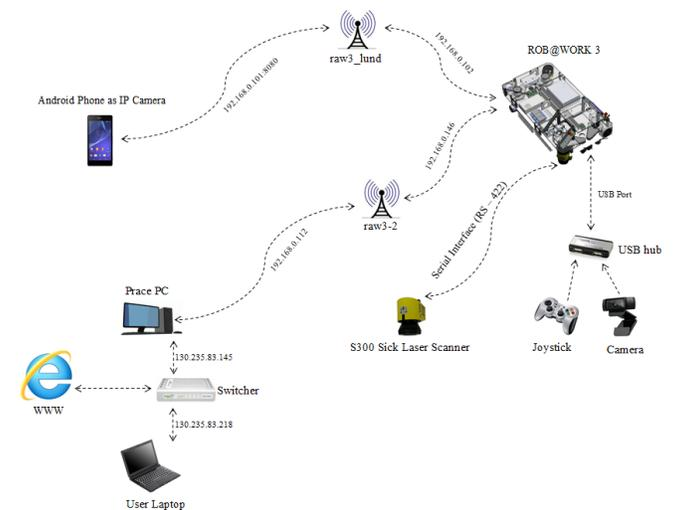
**Figure 2** The developed software and hardware architecture for the docking task (Alijani, 2016).
