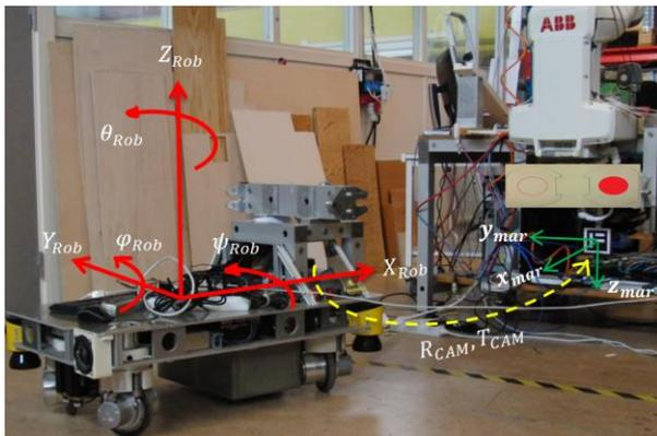
**Figure 1** The mobile robot Rob@work 3 and the docking platform under investigation (Alijani, 2016).
