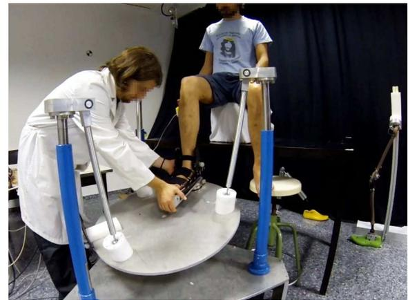
**Figure 20.** An example of using DMPs for teaching passive exercises for ankle rehabilitation (Abu-Dakka et al. 2015b, 2020).
