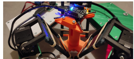
Figure 14. End effector (orange structure) and the crazyflie board with the Lighthouse deck
