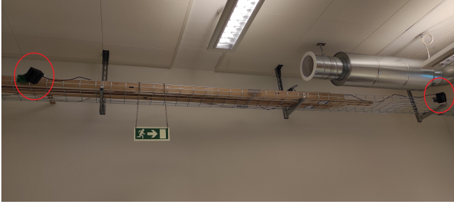
Figure 16. Beacons positioned in a rail with an 45 degrees angle facing downwards to map the room area in 3D
